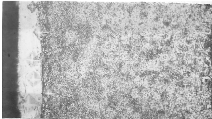
Fig. 8. Microstructure of nickel EEA surface layers after ball burnishing D_{\text{ш}} = 10 \text{ mm} , P_{\text{sp}} = 2060 \text{ MPa} \times 400
