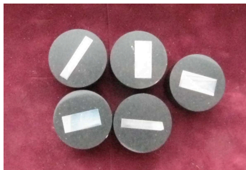
Fig. 4. Sections for metallographic and durometric tests
