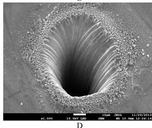
Fig. 4. View of traces of the impact of a picoseconds laser beam on C45, power
