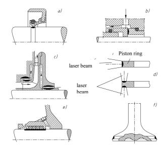
Fig. 2. Examples of using laser texturing in sealing technology (blackened places of laser treatment): a) pair with elastomeric seal, b) face seal, c) seal of a pump impeller, d) piston rings of piston pumps, e) sleeve of gland seal, f) faces of piston pump valves
