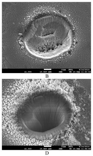
Fig.5. View of traces of the impact of a picoseconds laser beam on SiC, power 100%, frequency 50 kHz, impact time
