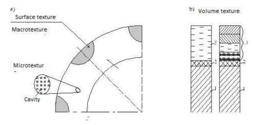
Fig.1. Model of textured surface layer: a) surface texture, b) volume texture; 1 – base, 2 – transitory layer, 3 – specific layers [5]
