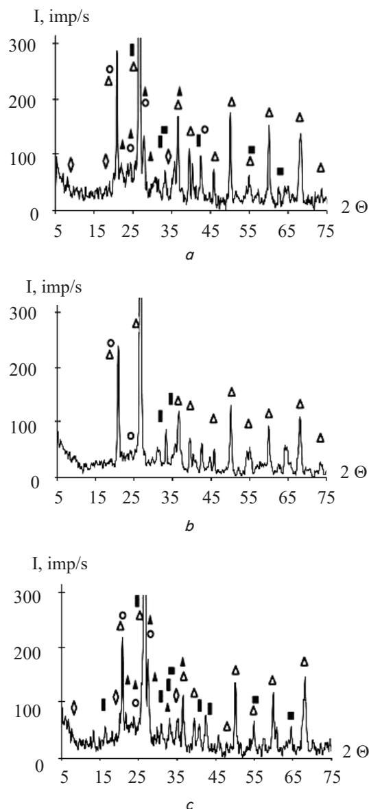
Fig. 17. Radiographs of samples of clinker bricks:
