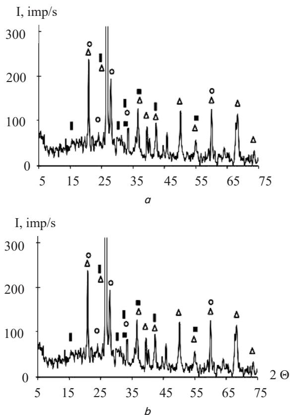
Fig. 13. Radiographs of samples of facing brick: *a* – sample No. 4; *b* – sample No. 6;  $\Delta$  –  $\beta$ -quartz;  $\circ$  – microcline;  $\mid$  – mullite;  $\diamond$  – biotite;  $\blacksquare$  – pyrite
