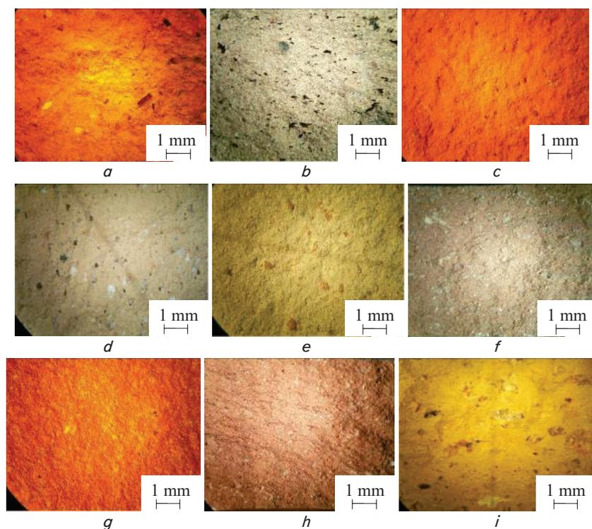
Fig. 2. Microstructure of the examined ceramic samples, reflected light: *a* – № 1; *b* – No. 2; *c* – No. 3; *d* – No. 4; *e* – No. 5; *f* – No. 6; *g* – No. 7; *h* – No. 8; *i* – No. 9
