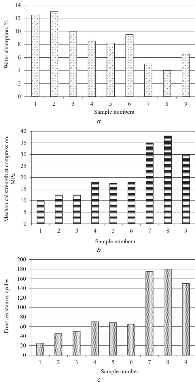
Fig. 1. Basic properties of the examined samples of ceramic bricks: a – water absorption, b – mechanical strength at compression, c – frost resistance
