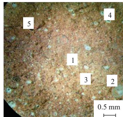
Fig. 12. Microstructure of sample No. 6, reflected light: 1 – main thermally altered clay glass-mass; 2 – grain of quartz; 3 – iron-containing mineral; 4 – finely dispersed residue from the decomposition of carbonates; 5 – pore
