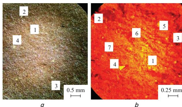
Fig. 14. Microstructure of sample No. 7, reflected light: *a* – magnification  $\times 32$  times; *b* – magnification  $\times 64$  times; 1 – main thermally altered clay glass-mass; 2 – grain of quartz; 3 – iron-containing mineral; 4 – grain of feldspar mineral; 5 – grain of artificial emaciator; 6 – grain of artificial marsh; 7 – pore
