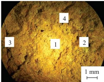
Fig. 3. Microstructure of sample No. 1, reflected light: 1 – main thermally altered clay mass; 2 – pore; 3 – microcrack; 4 – inclusion of an iron-containing mineral
