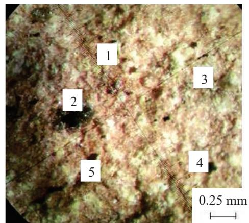
Fig. 6. Microstructure of sample No. 2, reflected light: 1 – main thermally altered clay mass; 2 – melted grain of sintering additive; 3 – grain of quartz; 4 – pore; 5 – iron-containing mineral
