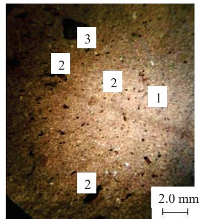
Fig. 5. Microstructure of sample No. 2, reflected light: 1 – main thermally altered clay mass, 2 – pore; 3 – impurities
