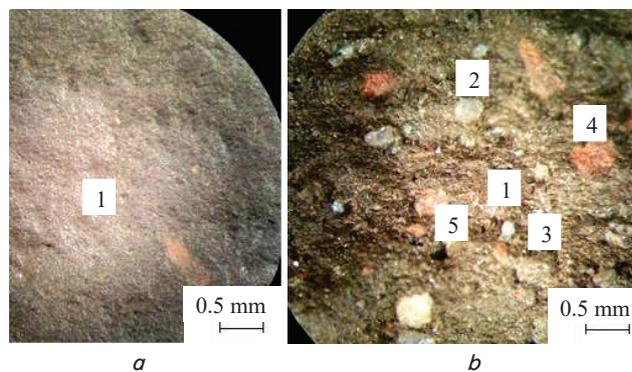
Fig. 15. Microstructure of sample No. 8, reflected light: *a* – external surface; *b* – inside the product; 1 – main thermally altered clay glass-mass; 2 – grain of quartz; 3 – grain of marsh; 4 – grain of artificial emaciator; 5 – pore
