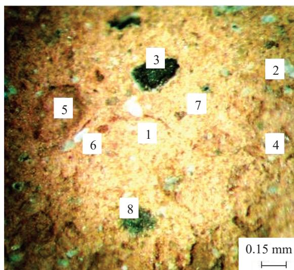
Fig. 9. Microstructure of sample No. 3, reflected light: 1 – main thermally altered clay glass-mass; 2 – grain (aggregate) of quartz; 3 – residue from the decomposition of carbonate; 4 – scale of mica; 5 – pore; 6 – iron-containing mineral; 7 – grain of artificial emaciater; 8 – grain of sintering additive
