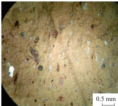
Fig. 10. Microstructure of sample No. 4, reflected light: 1 – main thermally altered clay glass-mass; 2 – grain of quartz; 3 – grain of feldspar mineral; 4 – scale of mica; 5 – iron-containing mineral, pore; 6 – grain of artificial emaciater; 7 – pore
