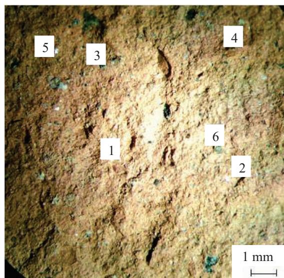
Fig. 8. Microstructure of sample No. 3, reflected light: 1 – main thermally altered clay mass; 2 – pore; 3 – grain of iron-containing mineral; 4 – finely dispersed carbonate residue; 5 – scale of hydromica; 6 – grain of quartz
