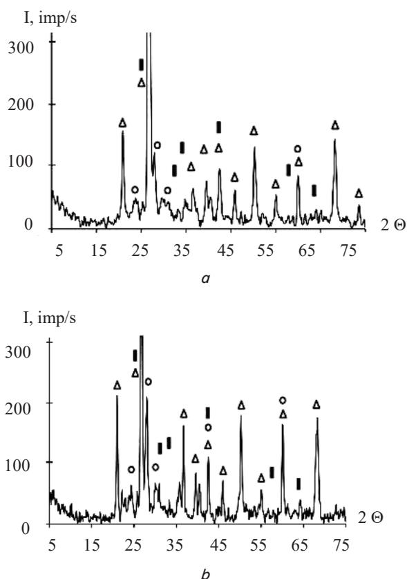
Fig. 7. Radiographs of samples of ordinary brick: *a* – sample No. 1; *b* – sample No. 2;  $\Delta$  –  $\beta$ -quartz;  $\circ$  – microcline; | – mullite
