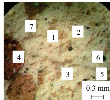
Fig. 11. Microstructure of sample No. 5, reflected light: 1 – main thermally altered clay glass-mass; 2 – grain of quartz; 3 – grain of feldspar mineral; 4 – pieces of broken products, 5 – iron-containing mineral, 6 – grain of artificial emaciater; 7 – pore
