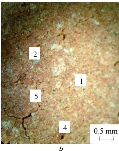
Fig. 4. Microstructure of sample No. 1, reflected light: *a* – inside the product; *b* – at the surface; 1 – main thermally altered clay mass; 2 – grain of quartz; 3 – inclusion of iron-containing mineral; 4 – pore; 5 – microcrack
