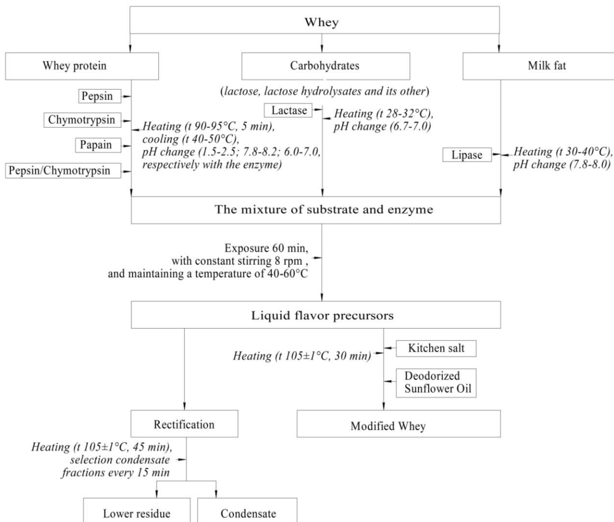
Fig. 1. Scheme of obtaining modified whey
