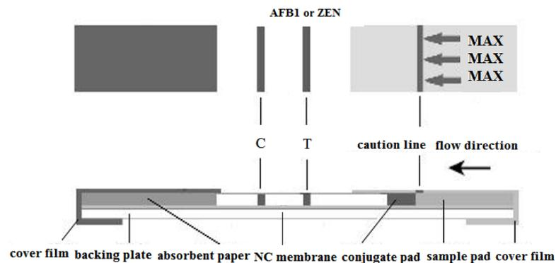
**Figure.3.36 The plane schematic diagram of single (AFB1 or ZEN) test strip.**
