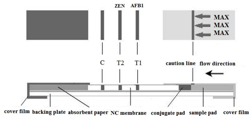
**Figure.3.37 The plane schematic diagram of dual AFB1 (or ZEN) test strip.**
