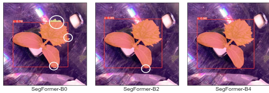
Fig. 57 Comparison of segmentation results. When CMFDR uses different size backbone networks, A, B, and C indicate that the CMFDR model is effective in predicting the same plant except when the SegFormer-B0, SegFormer-B2, and SegFormer-B4 backbone networks are used to visualize the same plant, respectively. The red and blue filters are the prediction results, and the white circle is added to emphasize the places with poor effect.
