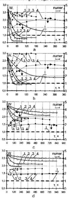
Fig. 1. Dynamics of the residual content phenolic compounds (W, %) in sunflower seed kernels with different size,  $\times 10^3$  m: 1 -(1-2), 2-(2-3), 3-(3-4), 4-whole, temperatures, °C:  $a - 80 \pm 2$ ,  $60 \pm 2$ ,  $c - 40 \pm 2$ ,  $d - 20 \pm 2$  and sensory evaluation of organoleptic characteristics of the samples, respectively - Ia, 2a, 3a, 4a. I reasonable range of phenolic compounds.
