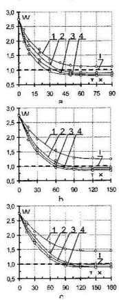
Fig. 2. Dynamics of residual phenolic compounds in fractionated crushed sunflower kernel with particles,  $\times$  10  $^3$  m: a - (1-2), b - (2-3), c - (3-4) after hydrothermal treatment at hydromodel: I - I : 5, 2 - I : 10, 3 - I : 15, 4 - I : 20 at  $60 \pm 2$  °C. I - reasonable range of phenolic compounds
