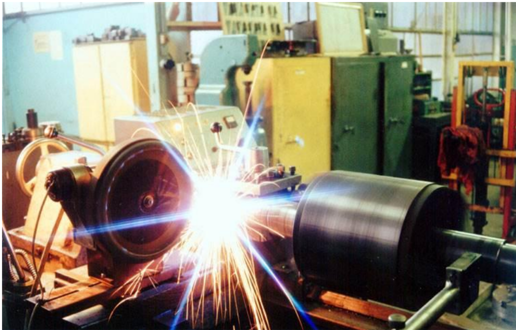
Fig. 6. Electroerosive alloying (EEA) of the rotor for the motor
