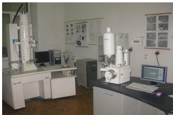
Fig. 2. Electric raster microscope (REM 106 I)
