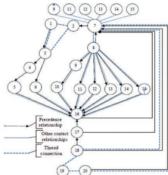
**Fig. 2. Graph of the planned sequence of dismantling a steam turbine for a virtual service system**
