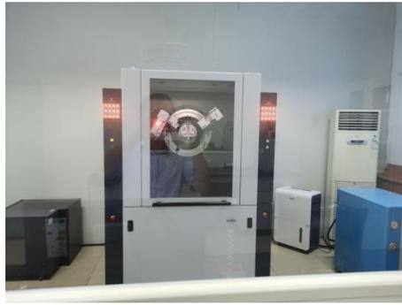
Figure 2.8 – The X-ray diffractometer (XRD)
