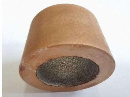
Figure 4.2 – Construction of running-in coatings on bearing bush surface
