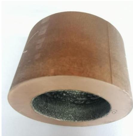
Figure 4.4 – Tin bronze bearing bush with running-in coatings after commissioning
