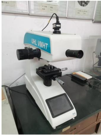
Figure 2.9 – The Microhardness tester
