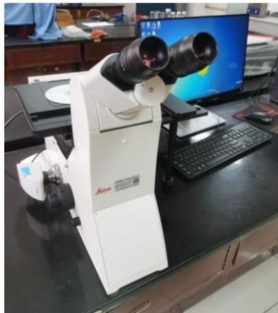
Figure 2.6 – The metallographic microscope
