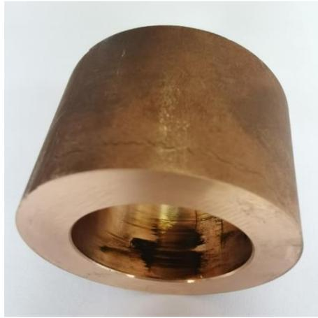
Figure 4.3 – Uncoated tin bronze bearing bush after commissioning
