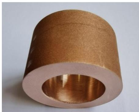
Figure 4.1 – Manufactured and preliminarily machined of bearing bush
