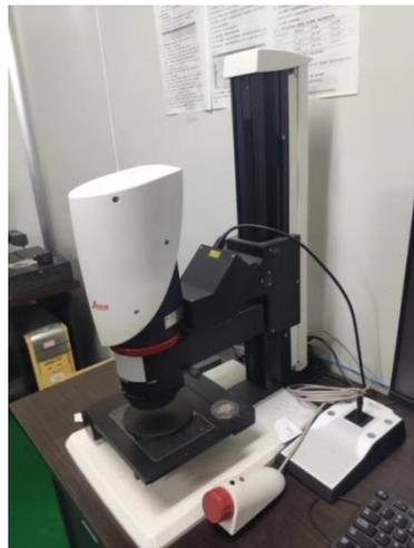
Fig. 2.9 – Super depth of field microscope
