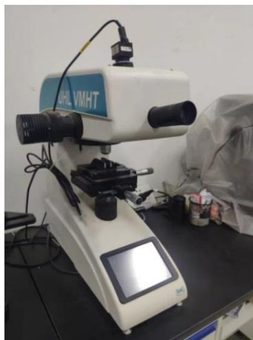
Fig. 2.7 – Vickers hardness tester
