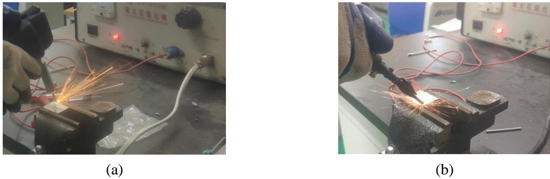
Fig. 3.39– Vibratory deposition process:a- conventional vibratory deposition;b- Pneumatic vibratory deposition
