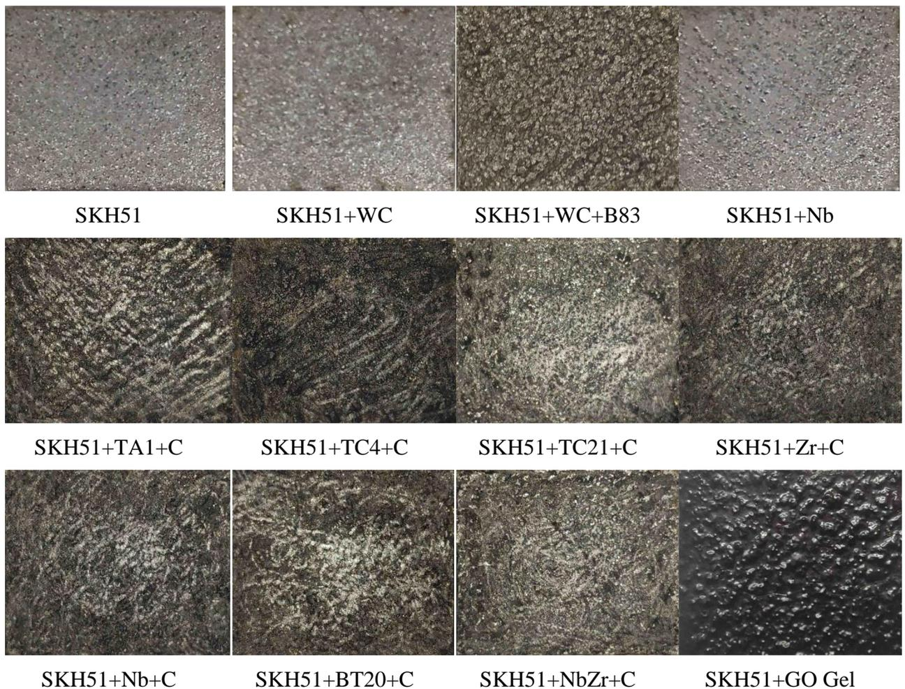
Fig. 3.24 – Surface topography of the treated coatings
