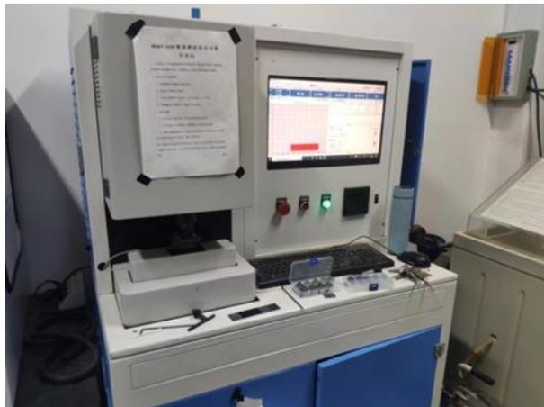
Fig. 2.8 – Linear reciprocating friction wear machine
