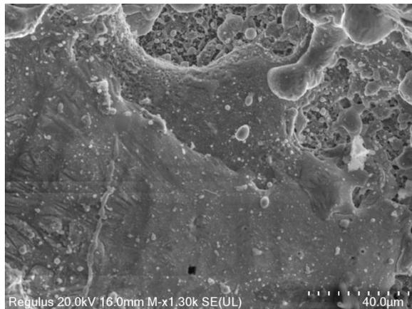
Fig. 3.31 – SEM of the B83 coating
