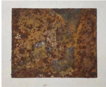
Fig. 4.4 – Surface corrosion morphology of 45 steel
