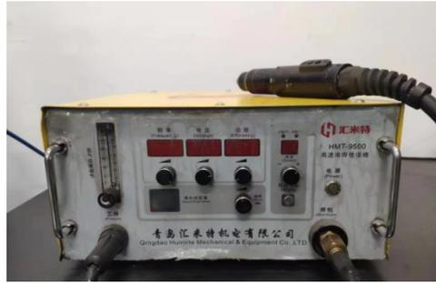
Fig. 3.1 – The high-speed ESD repair machine (HMT9500)
