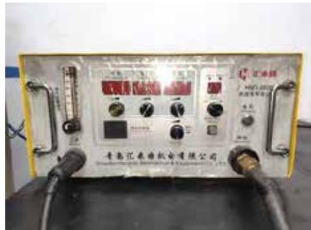
**Fig. 1. The electro-spark deposition equipment (HMT9500)**
