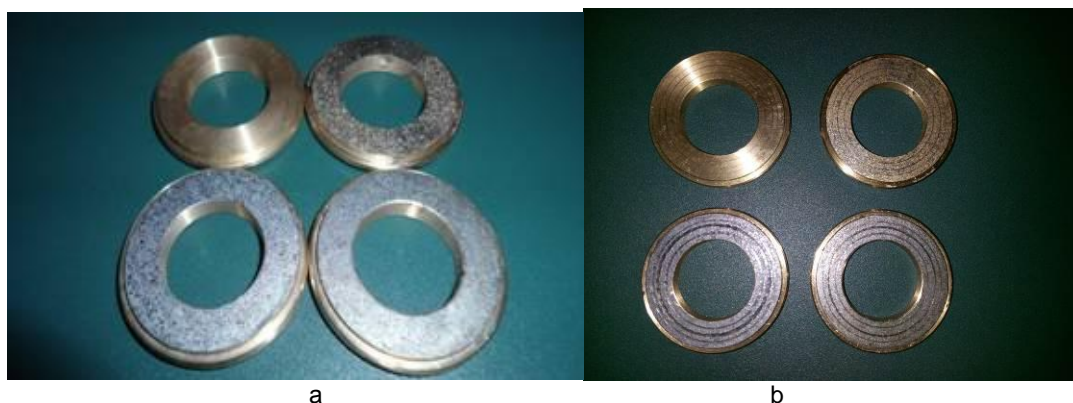
Fig. 2. Bronze specimen before (a) and after (b) testing
