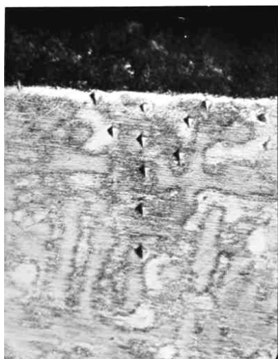
Fig.7. The microstructure and microhardness distribution of the surface layer of the specimen made of bronze OCS 5-5.
