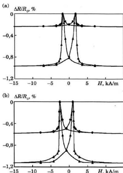
**Fig. 2:** Dependence of the longitudinal (•••) and the transverse (▲▲▲) MR versus the external magnetic field strength for the fresh-condensed three-layer CoNi/Ag/FeNi structure ( $d_{CoNi}=30$  nm,  $d_{Ag}=5$  nm,  $d_{FeNi}=30$  nm), temperature of measurements: 300 K(a), 150 K(b)
