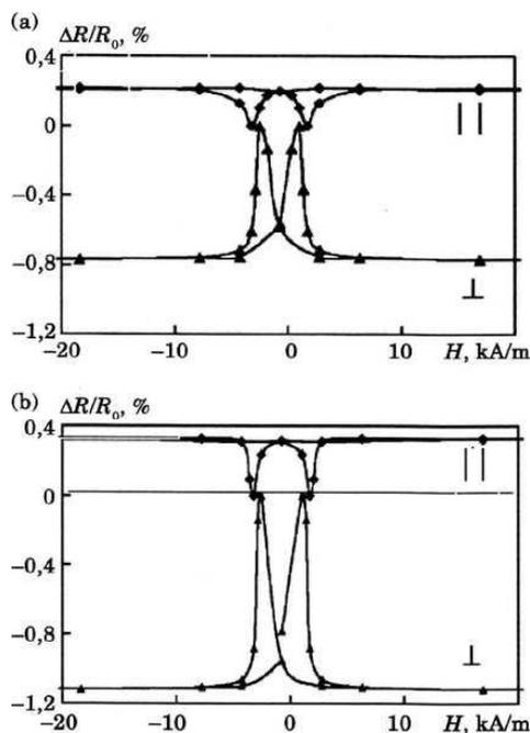
Fig. 4: Dependence of the longitudinal (||) and the transverse (⊥) MR versus the external magnetic field strength for the annealed at 700 K three-layer CoNi/Cu/FeNi structure; temperature of measurements: 300 K (a), 150 K (b)
